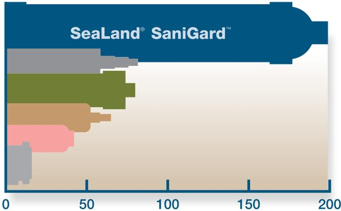
Chart indicates calculated capacity in grams of carbon disulfide that are adsorbed by each laboratory-tested\* vent filter. Based on this data, SeaLand SaniGard vent filters will outlast competitive filters by factors of 2.4 to 12.6 times longer.
